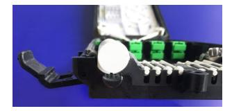
2. Drop cable sealing accessory for seal drop cable port if don't need use all of them
